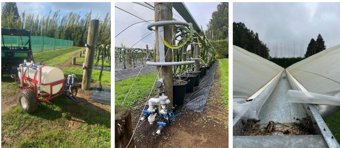
Figure 2. Portable fertigation unit (left); junction for connecting portable irrigation unit (middle); and channels that drain water that can be walked along to facilitate maintenance (right).
